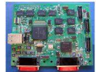
Flight Computer with Integrated Actuation Control
