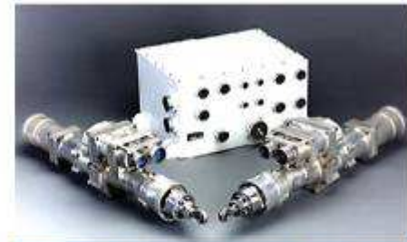
Atlas Electromechanical Thrust Vector Control Actuation System
