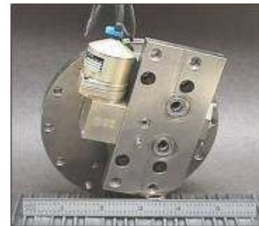
Divert and Attitude Control System Thruster Valves and Assemblies
